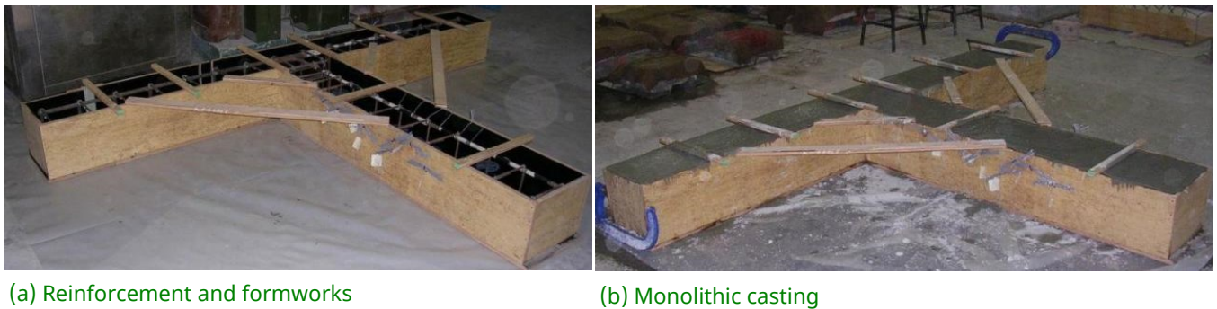
Figure 3. Preparation of specimen RC0
