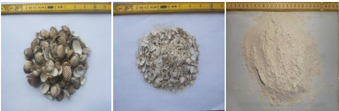
Figure 1. Seashells were cleaned, crushed and ground into fine particles.
