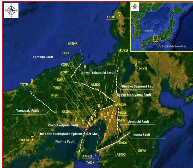
Figure 1. Location of seismic stations, earthquake epicentre, and active faults (modified from Google Earth (2018))
