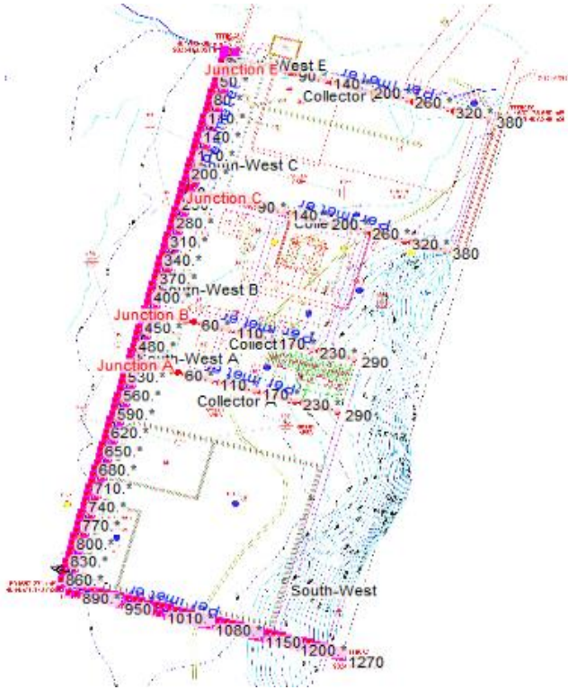
Figure 4. Flow simulation for south-west perimeter drainage channel and all of the collector-drainage channels.
