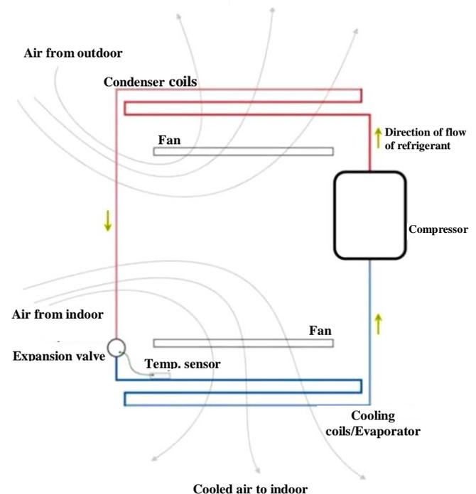
Figure 1. Principle Mechanism of Air Conditioning (Talat, 2016).
