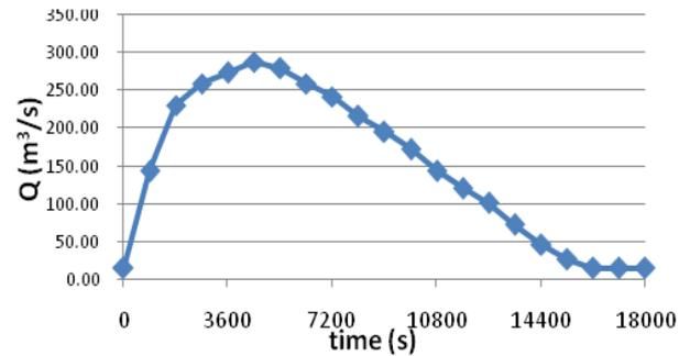
Figure 6. Hydrograph of Debris Flow
