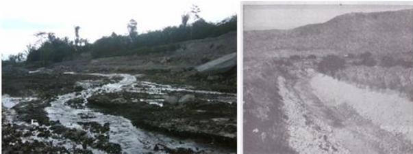
Figure 5. Photo of Putih River (left) compared with one of photos from U.S Geological Survey (right) to determine Manning value
