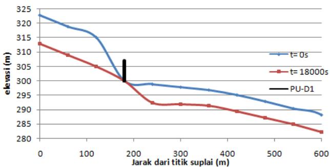
Figure 12. River Bed Level (Distance from supply point 0-600 m) – Scenario II
