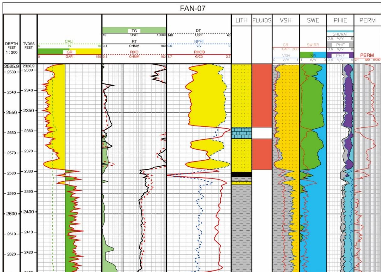
FIGURE 3. Lithology and fluid determinations from FAN-07.
