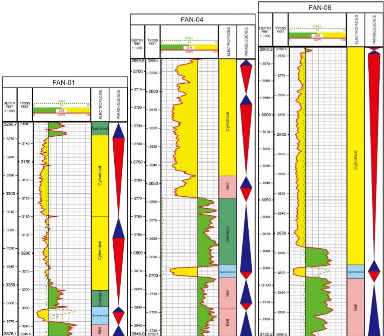
FIGURE 4. Electrofacies and parasequence result of FAN-01, FAN-04, and FAN-06.
