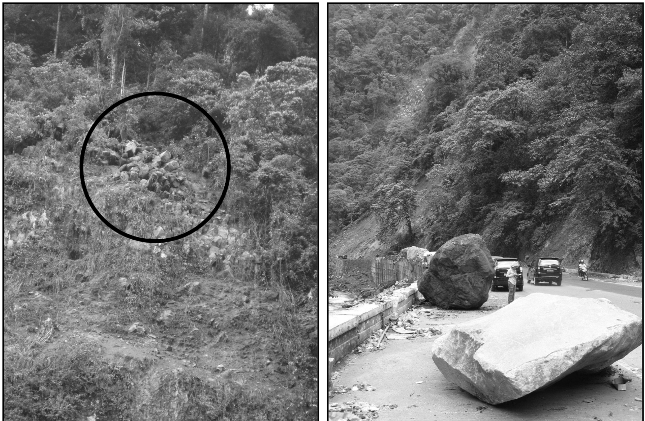
Figure 3: (a) Andesitic materials that are still hanging in the top of slope; (b). A big andesite boulder from the rockfall
