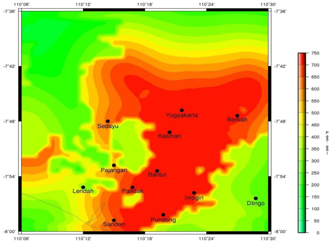
Figure 12: Seismic hazard maps expressed in pga (gal) for 500 years return interval.
