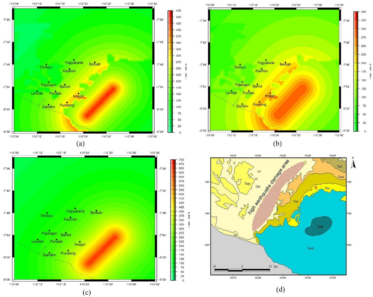
Figure 7: PGA map of the 27, May 2006 Yogyakarta earthquake by using the attenuation relationship of (a) Takahashi *et al.*, 2000, (b) Boore *et al.*, 1997, (c) Fukushima & Tanaka, 1990 and (d) Map showing the most earthquake damage area to correlate with the resulted PGA values.
