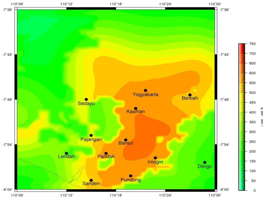
Figure 10: Seismic hazard maps expressed in pga (gal) for 100 years return interval.
