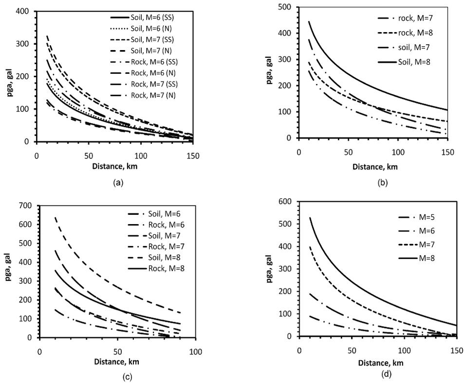
Figure 3: Variation of peak ground acceleration (PGA) with source distance for attenuation relation of (a) Boore *et al.*, 1997, (b) Youngs *et al.*, 1997, (c) Fukushima and Tanaka, 1990 and (d) Takahashi *et al.*, 2000.
