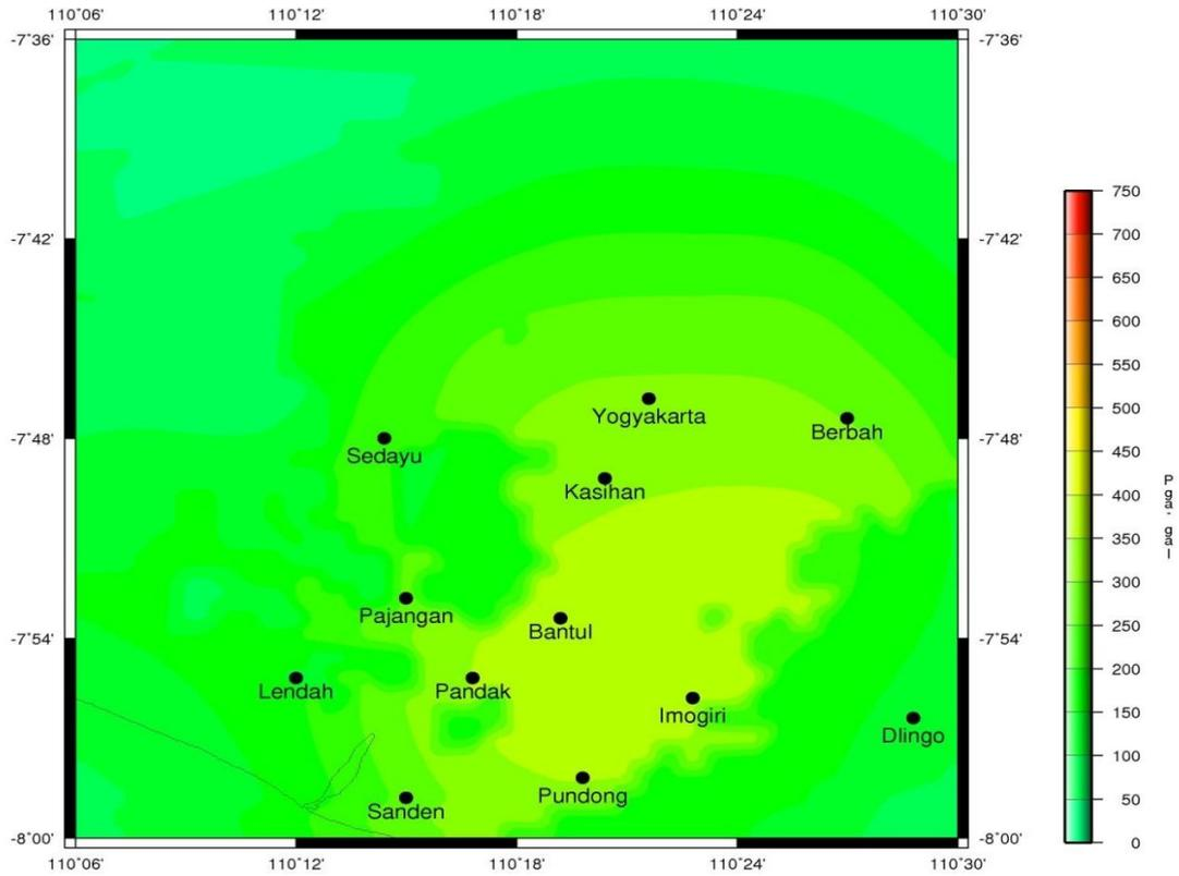
Figure 8: Seismic hazard maps expressed in pga (gal) for 10 years return interval.
