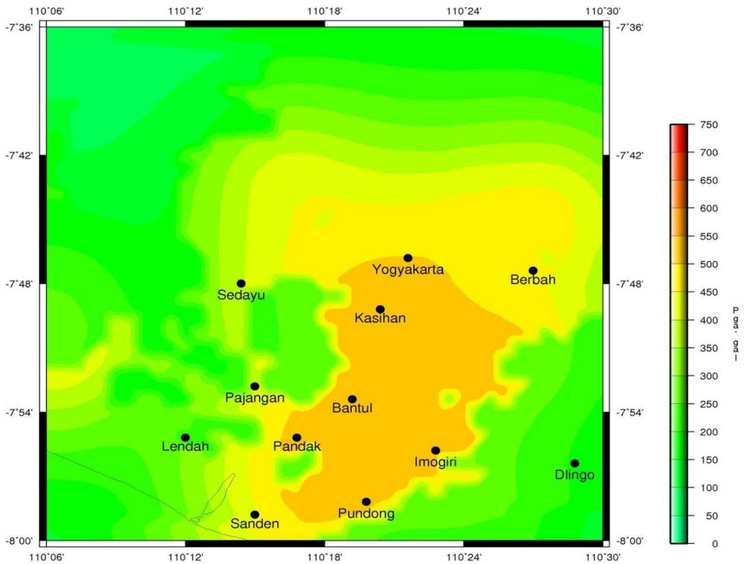
Figure 9: Seismic hazard maps expressed in pga (gal) for 50 years return interval.
