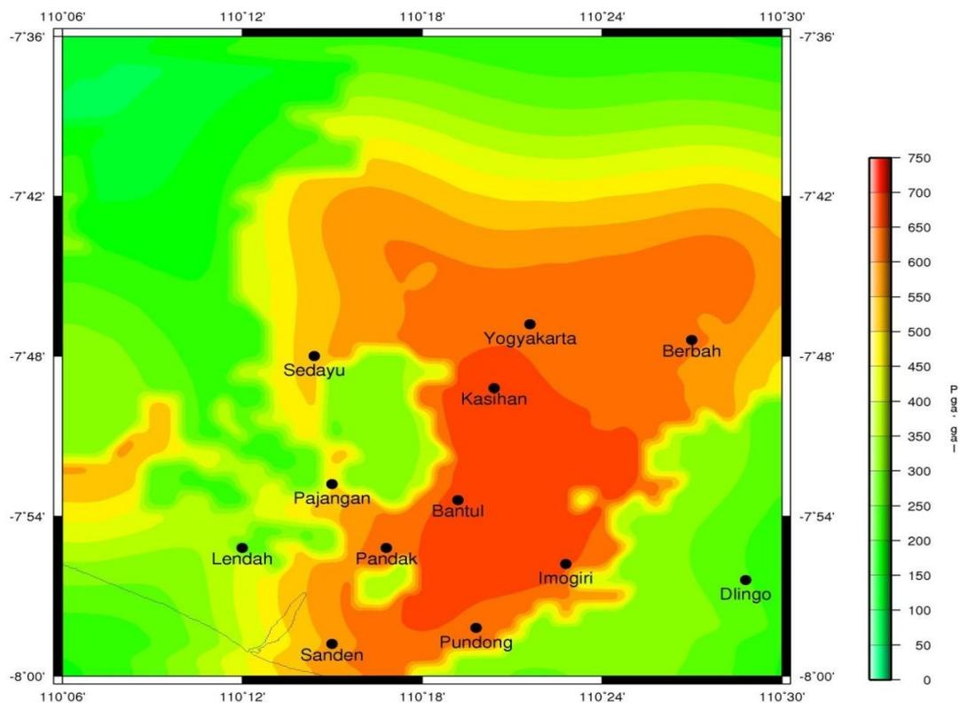
Figure 11: Seismic hazard maps expressed in pga (gal) for 200 years return interval.
