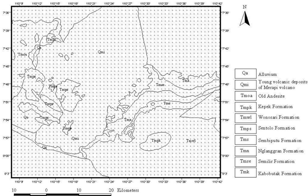
Figure 6: Geological map of Yogyakarta area showing the grid points in  $0.01^\circ \times 0.01^\circ$  interval where the peak ground acceleration values are estimated.
