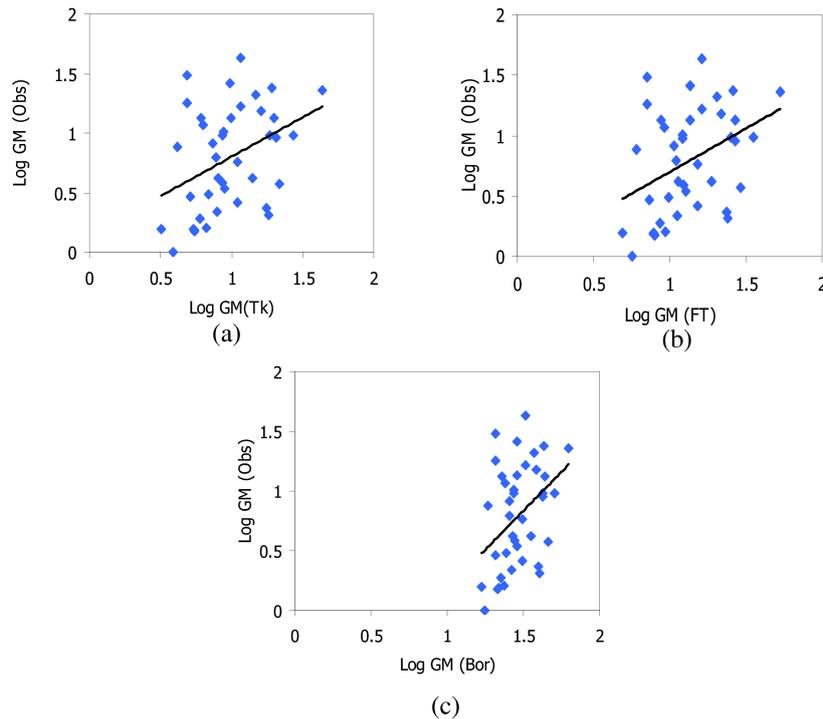
Figure 5: The plots of observed ground motion parameters; GM(Obs) against the resulted ground motion parameters using (a) Takahashi *et al.*, 2000 ( GM (Tk)), (b) Fukushima and Tanaka, 1990 (GM (FT)) and (c) Boore *et al.*, 1997 (GM (Bor)).
