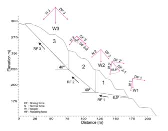
Figure 7: Geometry of cross section A and forces acting on rock mass blocks above failure surfaces assigned in PF method.
