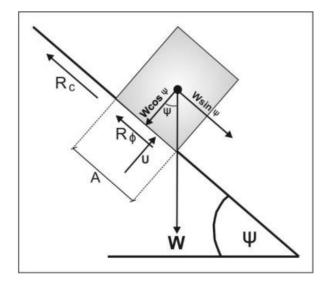
Figure 1: Forces acting on a failure surface of rock slope (González de Vallejo and Ferrer, 2011).
