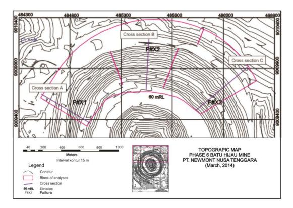
Figure 5: Locations of rock slope failures and cross sections for slope stability analyses.
