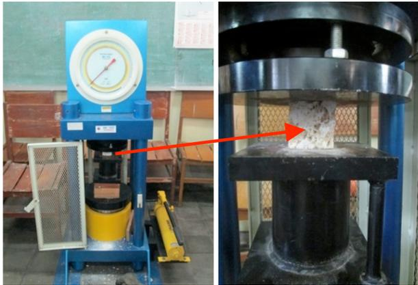
Figure 6: Uniaxial Compressive Strength (UCS) equipment.
