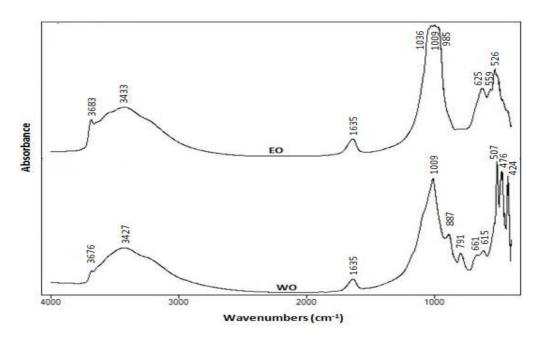
Figure 4: Infrared spectra of west ore (WO) and east ore (EO) samples used in the experiment
