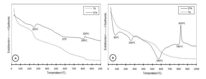
Figure 3: TG/DTA curves of ore sample (WO) from Soroako west block (A) and east ore (EO) from Petea area (B)
