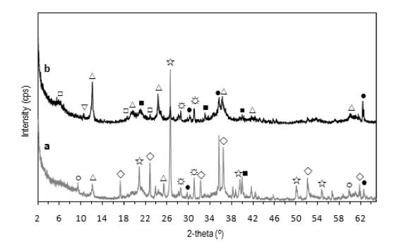
Figure 2: X-ray diffraction patterns of saprolitic ore samples from Soroako west block (a) and Petea area (b). Notes: + = serpentine (lizardite),  $\star$  = quartz,  $\Box$  = chlorite, • = maghemite/magnetite,  $\diamondsuit$  = forsterite,  $\bigcirc$  = talc,  $\diamondsuit$  = enstatite,  $\nabla$  = amphibole
