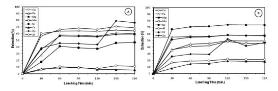
Figure 7: Graphs showing the percentage of metals extraction from Soroako Ni-laterite ores under different leaching time. A: West ore sample (WO), and B: East ore sample (EO)
