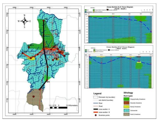
FIGURE 3. Surface and sub-surface lithology in the study area.
