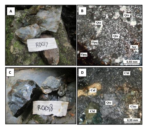
Figure 3: Outcrop/handspecimen and petrographic microphotograph of altered wall rocks in Rampi block prospect: (A) and (B) silicified rock; (C) and (D) propylitic altered rock.
