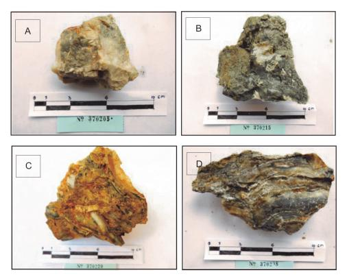
Figure 4: Types and textures of chalcedonic-quartz vein containing significant gold found in Rampi block prospect, North Luwu district: (A) Massive chalcedonic quartz vei, (B) Brecciated quartz vein, (C) Brecciated and oxidized (limonitized) quartz vein, and (D) Laminated chalcedonic quartz vein.
