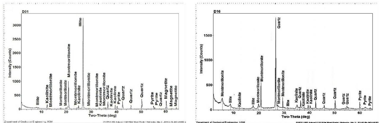
Figure 7: X-Ray Diffraction patterns of altered andesitic tuff from the Pelangan area.
