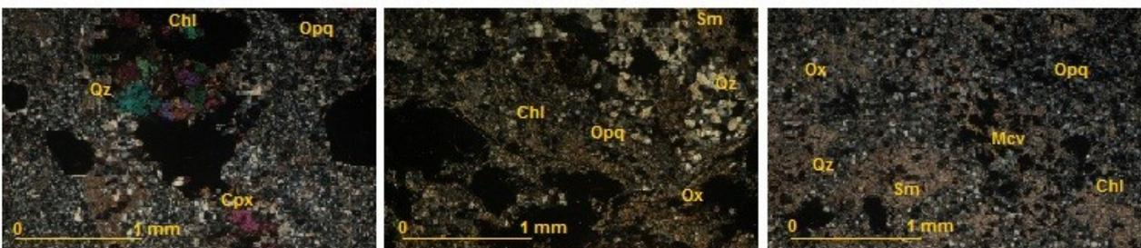
Figure 5: Optical photomicrographs of altered andesitic tuff showing the presence of clinopyroxene (Cpx), quartz (Qz), opaque mineral (Opq), chlorite (Chl), smectite (Sm), iron oxides (Ox), and muscovite (Mcv).
