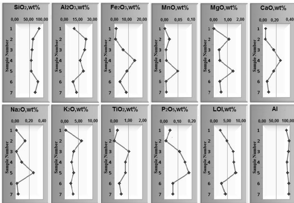
Figure 8: Vertical variations in the geochemical composition and alteration intensity of altered andesitic tuff.
