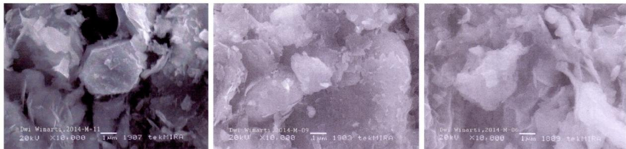
Figure 6: SEM images of altered andesitic tuff showing the presence of hexagonal plate of kaolinite and rosette of quartz (left), flake of kaolinite (middle), and flake of quartz and rolled plate of kaolinite (right).
