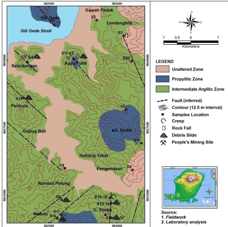
Figure 3: Hydrothermal alteration zone map of Pelangan area.
