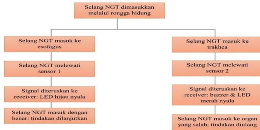
Gambar 2. Alur Sistem Smart Sensor NGT
