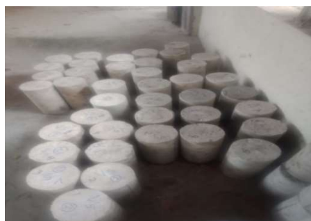
Gambar 2. Perawatan sampel beton (disiram/ditutup karung goni)
