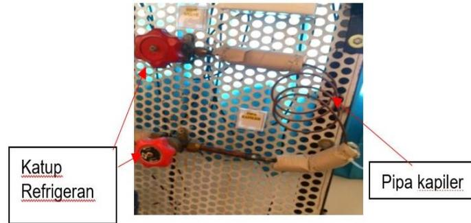
Gambar 2. Pipa Kapiler AC Trainer Unit
