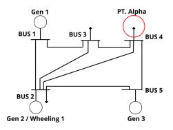
Fig. 3 Test system of 5-bus test.
