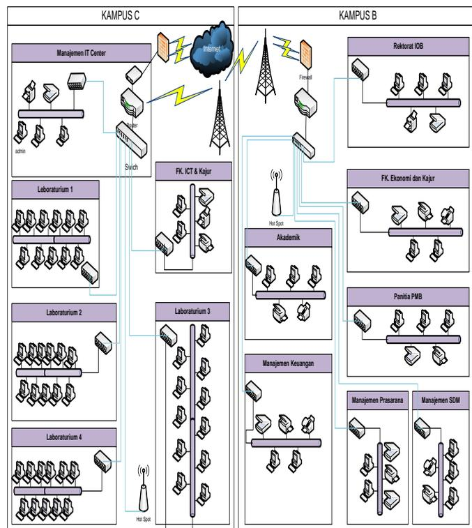
Fig. 8 Network architecture scheme.
