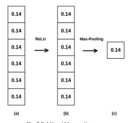
Fig. 7 ReLU and Max-pooling processes.
