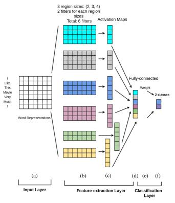
Fig. 3 CNN architecture.
