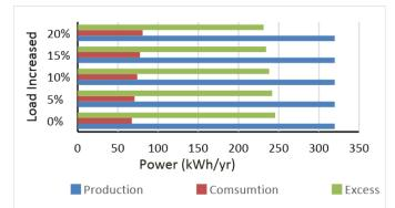
Fig. 6 Comparison of total electricity production, total electricity consumption, and excess electrical energy generated from load growth.
