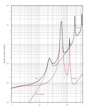
Fig. 1 Characteristics of atmospheric attenuation.
