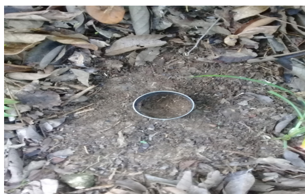
Figure 19. Soil pedestal in the land unit L4c4B with shrub land use. Soil loss by field indicators was 18,44tons/ha/yr, and by RUSLE was 63,82tons/ha/yr. Land degradation rate by erosion was categorized low to high.
