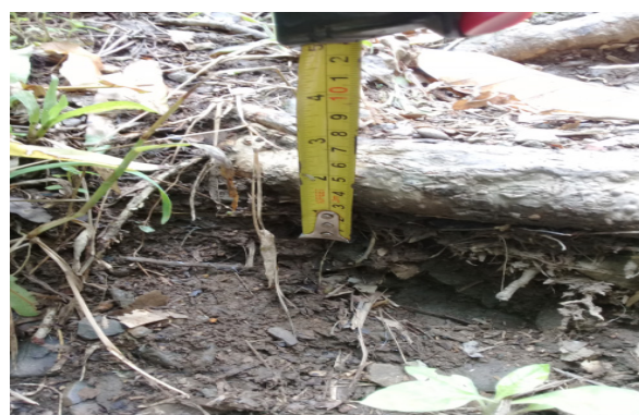
Figure 20. Exposed roots in the land unit L5c3B with shrub land use. Soil loss by field indicators was 34,99tons/ha/yr, and by the RUSLE was 1218,18tons/ha/yr. Land degradation rate by erosion was categorized moderate to high
