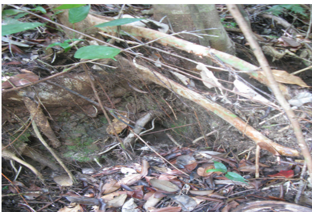
Figure 11. Exposed tree roots in land unit L0c5B with shrub land use. Soil loss by field indicator was 24,42tons/ha/yr, and by RUSLE was 33,22 t/ha/yr. Land degradation rate by erosion was categorized moderate.
