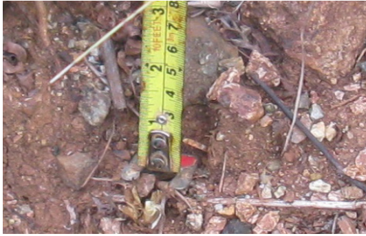
Figure 15a. Soil pedestal and gully in land unit L3c3B with shrub land use. Soil loss by field indicators was 107.46tons/ha/yr, and by RUSLE was 431,44tons/ha/yr. Land degradation rate by erosion was categorized high to very high.
