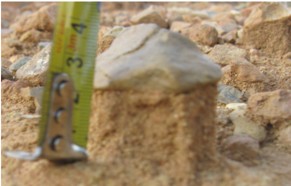
Figure 16. Soil pedestal and rill in the land unit L3c5A with settlement land use. Soil loss by field indicators 675.62tons/ha/yr, and by RUSLE was 1882.26tons/ha/year. Land degradation rate by erosion was categorized very high.
