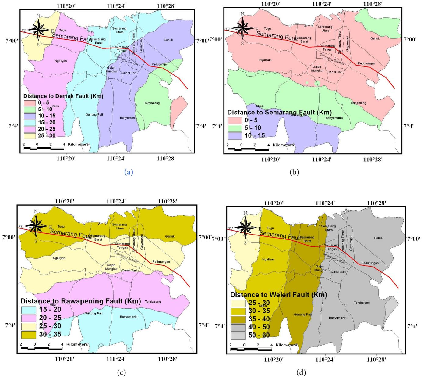
Figure 6. Earthquake source distance distribution maps of Semarang (a), Demak (b), Rawapening (c) and Weleri (d) fault lines.
