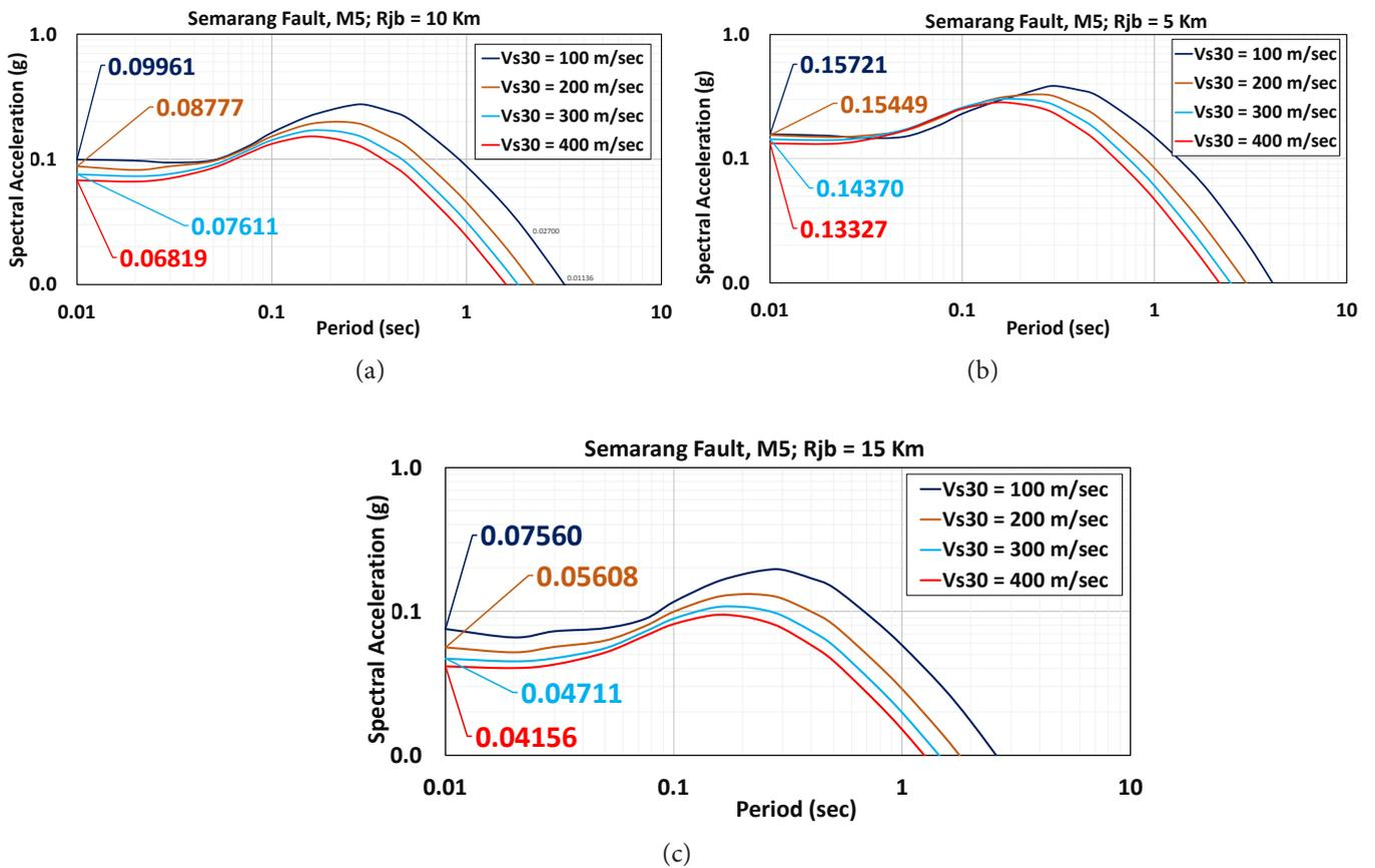
Figure 8. Surface spectral acceleration calculation of four GMPE due to the Semarang fault earthquake scenarios at Rjb = 5 km (a), Rjb = 10 km (b) and Rjb = 15 km (c).
