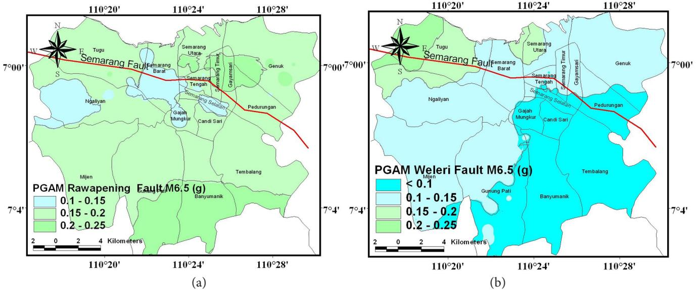
Figure 12. PGAS distribution map of Rawapening (a) and Weleri (b) fault earthquake scenarios with a magnitude of M6.5.
