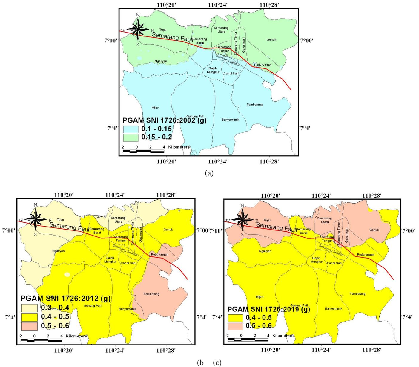
Figure 9.  $PGA_M$  distribution maps of SNI 1726:2002 (a), SNI 1726:2012 (b) and SNI 1726:2019 (c).
