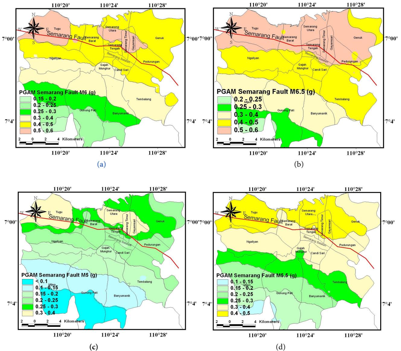
Figure 10. PGAS distribution map of Semarang fault earthquakes at M6.5 (a), M6 (b), M5.5 (c) and M5 (d).
