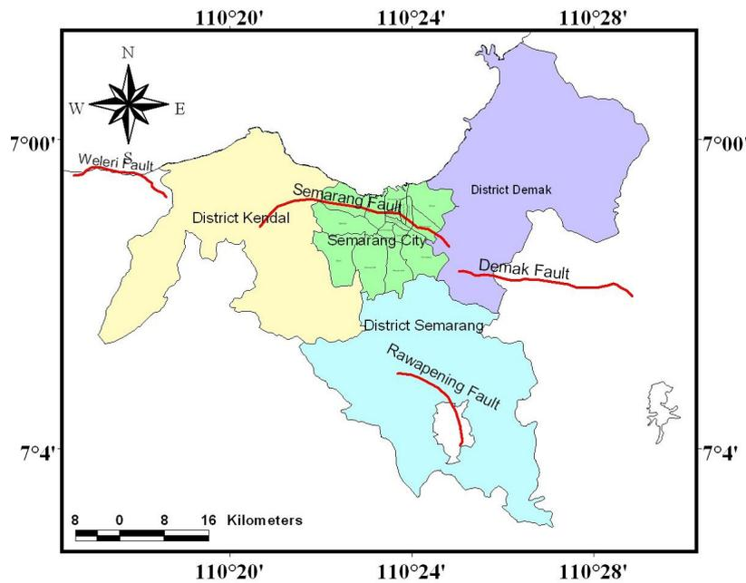
Figure 1. Fault lines around the city of Semarang
