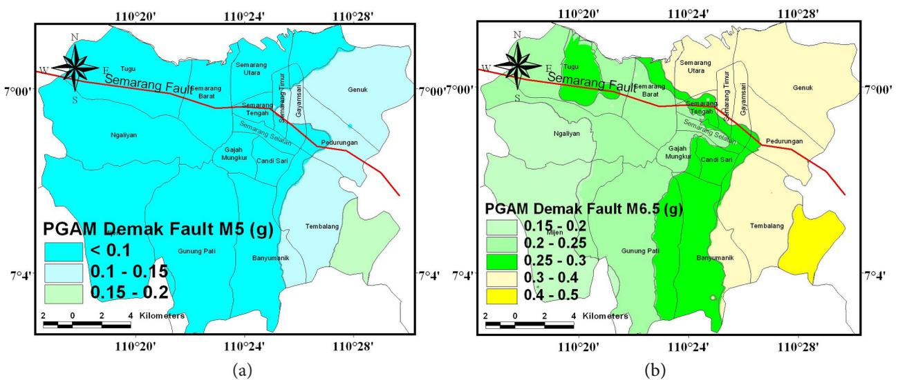
Figure 11. PGAS distribution map for Demak fault earthquake magnitudes of M6.5 (a) and M5 (b).
