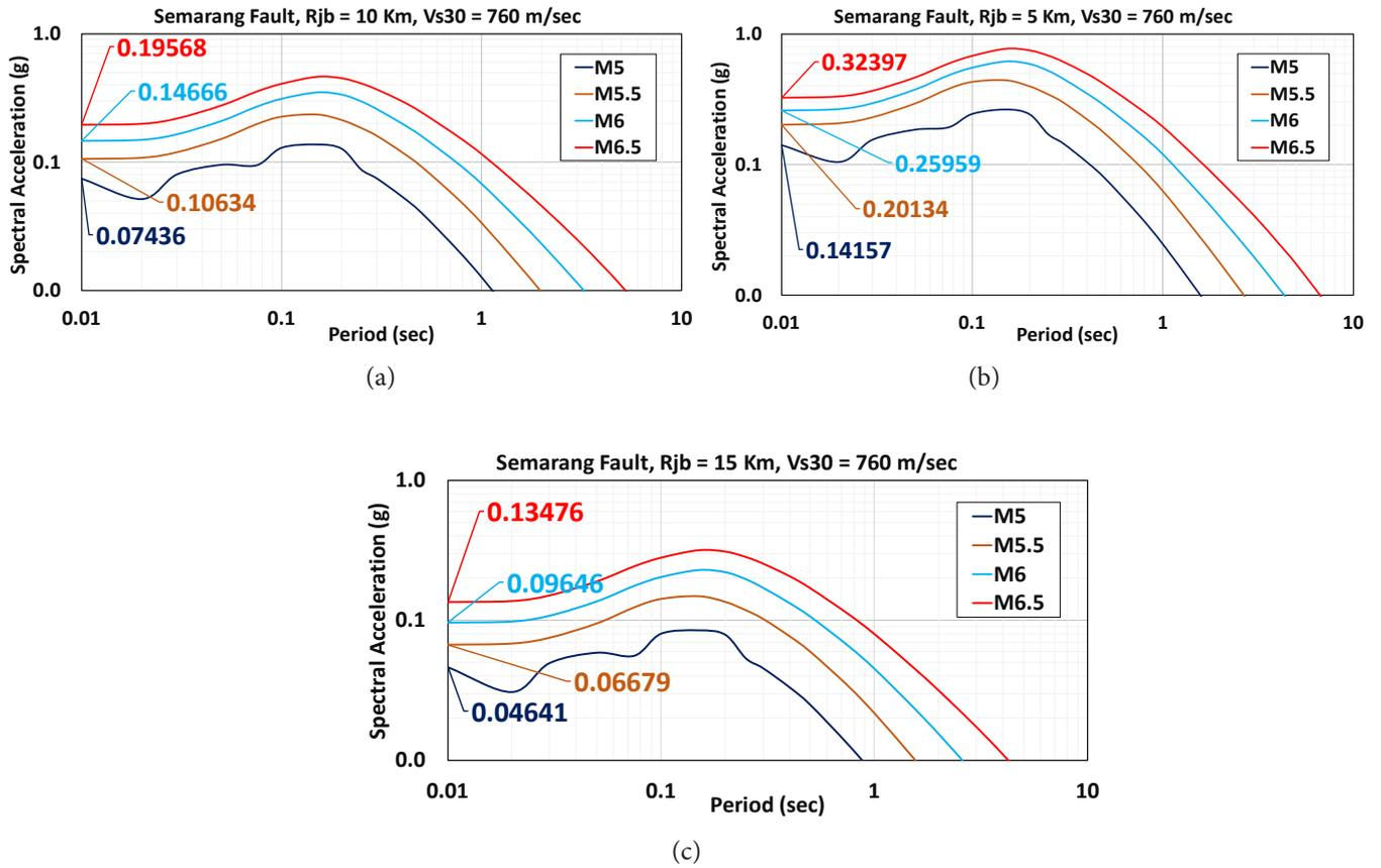
Figure 7. Spectral acceleration calculation of four GMPEs due to the Semarang fault earthquake scenarios at Rjb = 5 km (a), Rjb = 10 km (b) and Rjb = 15 km (c).
