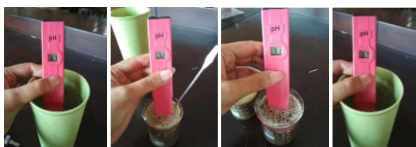
Figure 6. Measurement of Four Point Location Water pH
