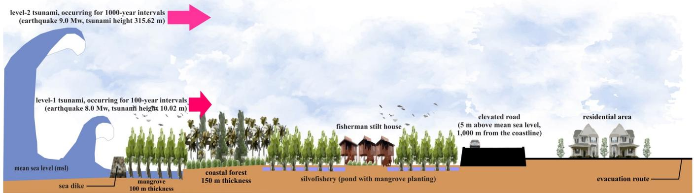
Figure 6. Conceptual Illustration of A Section of A New Approach of Tsunami Mitigation Strategies to Reduce The Risk of Tsunami Disasters and To Optimize The resources Through The Multi-Layer Defence Systems
