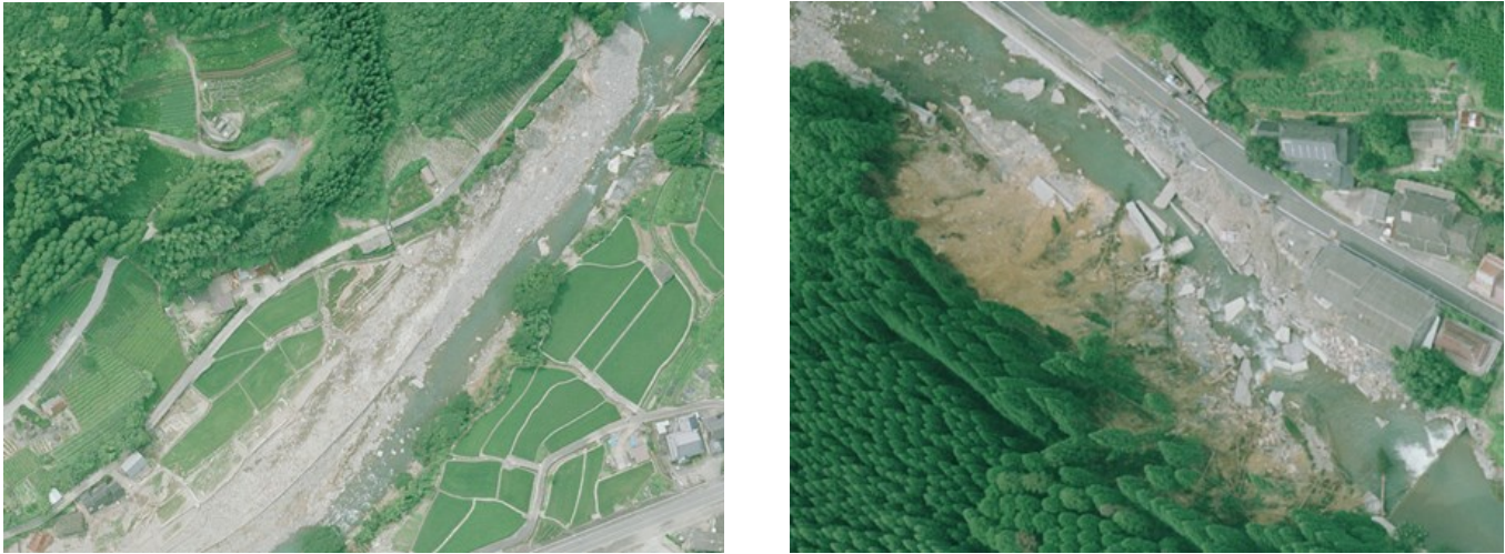
Figure 18. Areal photos show woody debris pieces in 'Ikenoyama' district as a production site and 'Ono' district as a deposition site.
