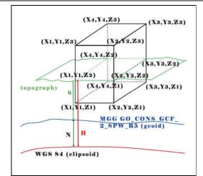
Figure 7. Geometric and orthometric heights in a 3D cadastre using GGM GO\_CONS\_GCF\_2\_SPW\_R5 hybrid geoid
