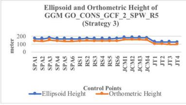
Figure 10. Comparison of ellipsoid and orthometric heights using GGM GO\_CONS\_GCF\_2\_SPW\_R5
