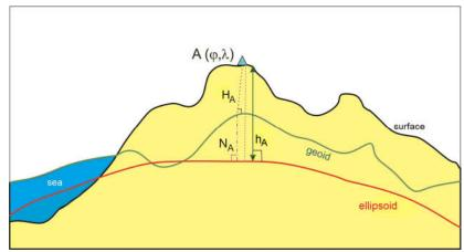
Figure 1. Geometrical relationship between ellipsoid, geoid and topographical surface (modified version from Featherstone *et al.*, 1998)
