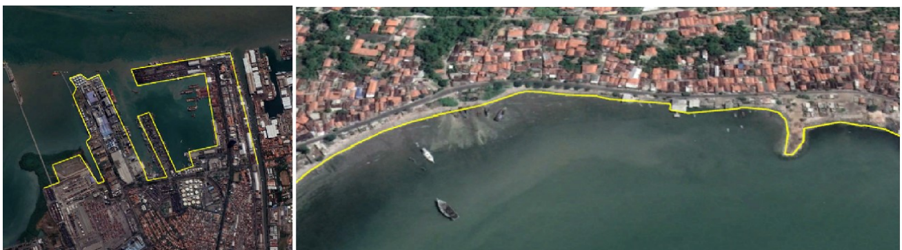
Figure 4. Digitizing of High-Water Level of Coastline in port (building) (left) and dry area (right) (Khomsin and Ayuningtyas, 2017)
