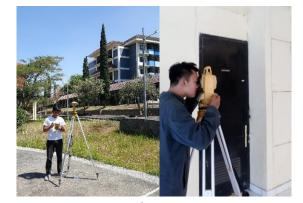
Figure 3. Control point measurements
