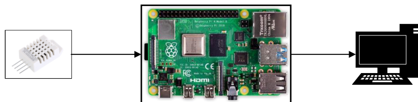
Figure 1 Weather Monitoring Hardware Design
