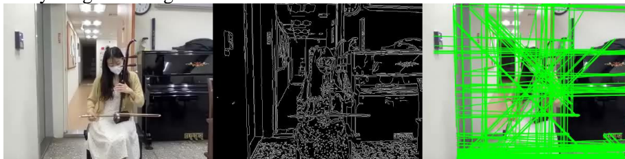
Figure 2.2 The Hough Line Algorithm Line Detection Result Before Image Processing
