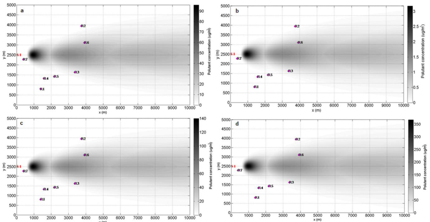
**Fig 4.** Dispersion of pollutant gases case 1(a) SO<sub>2</sub>, (b) CO, (c) NO<sub>2</sub>, (d) TSP
