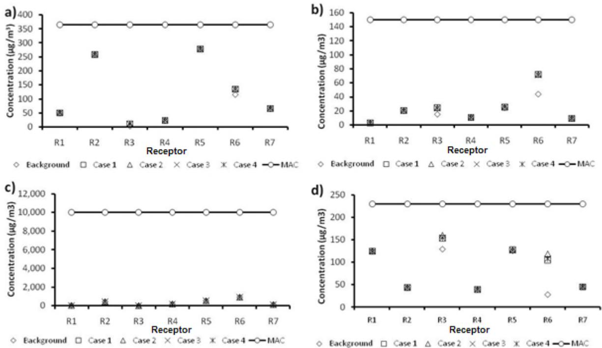
**Fig 3.** Pollutant gas concentration into the receptor (a) SO<sub>2</sub>, (b) CO, (c) NO<sub>2</sub>, (d) TSP (Note: Maximum Allowable Concentration is based on Indonesian Government Regulation No. 41 1999)
