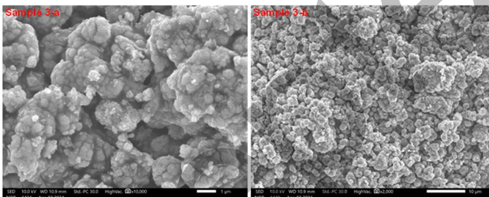
Fig 8. SEM images of the high-grade TiO<sub>2</sub> samples at NaOH concentration (800 g/L)
