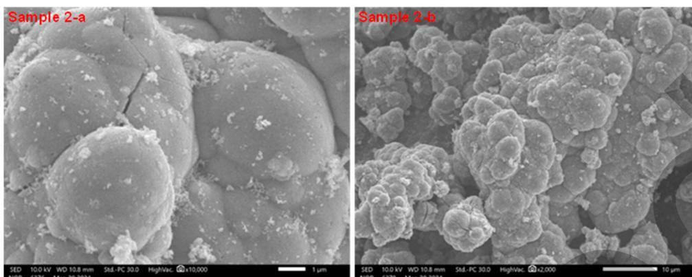
Fig 7. SEM images of the high-grade TiO<sub>2</sub> samples at NaOH concentration (600 g/L)
