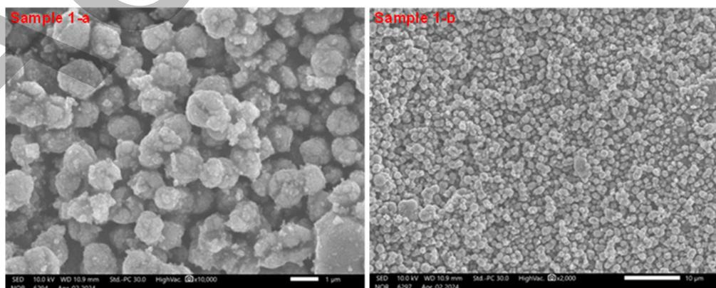
**Fig 6.** SEM images of the high-grade  $\text{TiO}_2$  samples at NaOH concentration (400 g/L)
