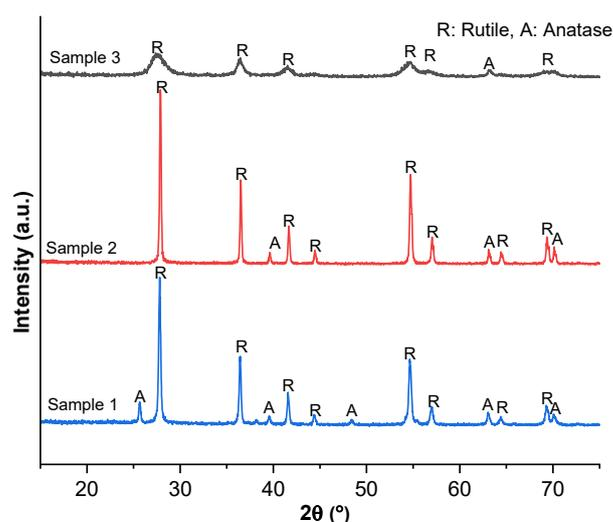
Fig 3. The XRD patterns of obtained three samples synthesized; sample 1: 400 g/L, sample 2: 600 g/L, sample 3: 800 g/L
