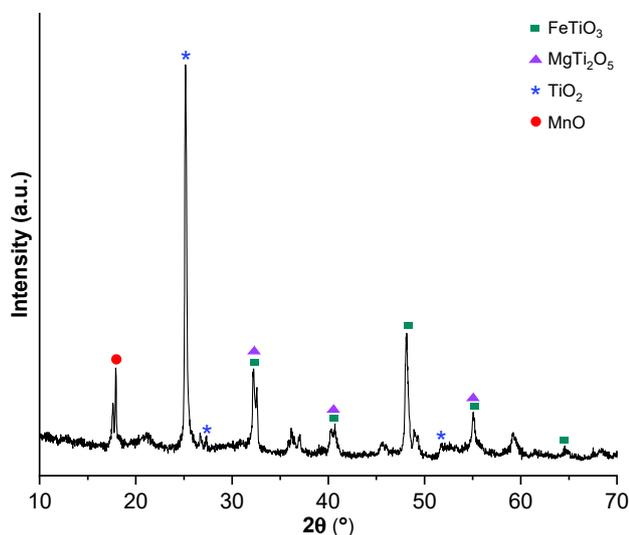
**Fig 1.** The XRD pattern of TS (ilmenite)
