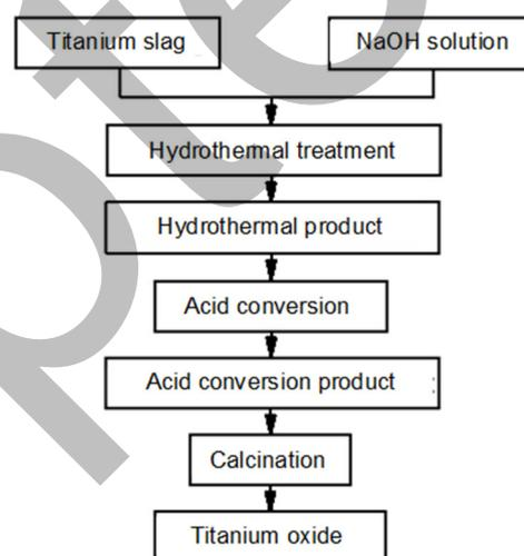
Fig 2. The flow chart of the titanium hydrothermal process
