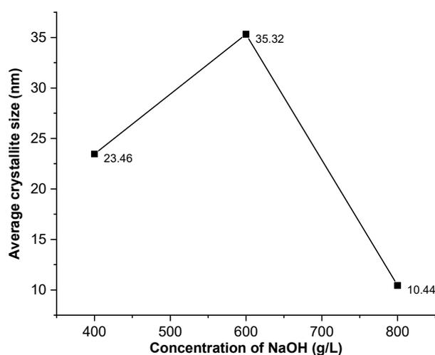
Fig 4. The average crystalline size of TiO<sub>2</sub>
