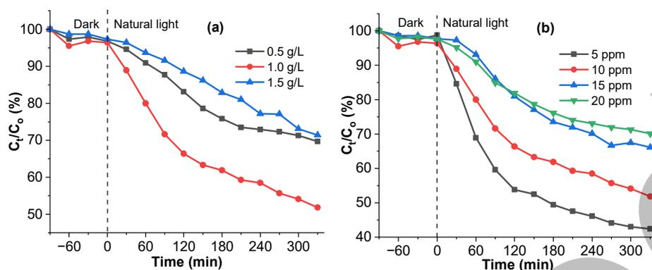
Fig 6. Photocatalytic activity of FSAC-2:1 with (a) different dosages and (b) different MB concentrations
