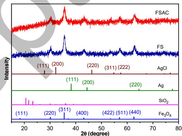
**Fig 1.** XRD patterns of FS and FSAC
