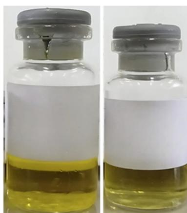
**Fig 8.** Pictures of feed (Left) and biojet fuel (Right) from palm cooking oil hydrotreatment
