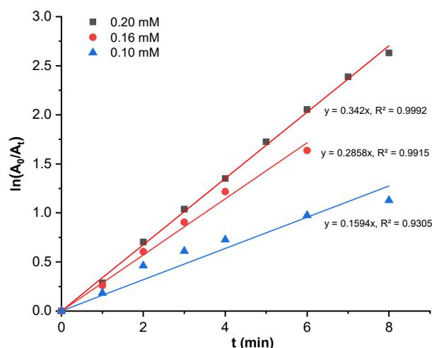
**Fig 6.** First-order plots for the decolorization of PS by UV/chlorine process at different chlorine concentrations. Experimental conditions: [PS] = 0.044 mM; pH = 4.22; T = 25 °C
