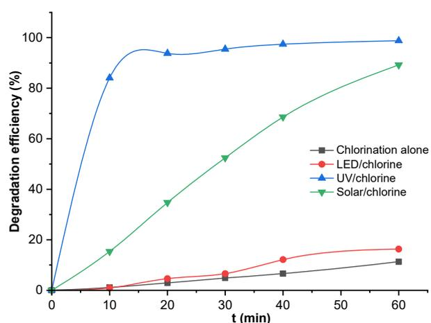
**Fig 8.** PS degradation by chlorination alone, UV/chlorine and sunlight/chlorine processes. Experimental conditions: [PS] = 60 mg/L; [chlorine] = 0.06 g/L; pH = 5.03.
