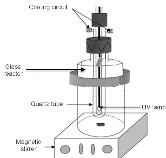
**Fig 2.** Experimental setup for the irradiation experiments
