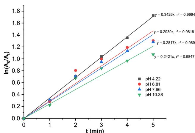
**Fig 5.** First-order plots for the decolorization of PS by UV/Chlorine process at different values of pH. Experimental conditions: [PS] = 0.044 mM; [Cl(+I)] = 0.2 mM, pH= 4.22–10.38; T = 25 °C
