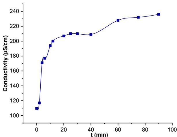
**Fig 9.** Evolution of conductivity during PS degradation using UV/chlorine process
