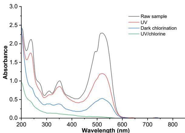
**Fig 4.** Changes in the UV-vis absorbance spectrum in PS dye solution during UV/chlorine process. Experimental conditions: [PS] = 0.044 mM; [chlorine] = 0.200 mM; pH = 7; T = 25 °C
