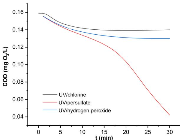
**Fig 10.** COD removal from the PS dye in AOP studied. Experimental conditions: [PS] = 0.044 mM; [H<sub>2</sub>O<sub>2</sub>] = [chlorine] = [S<sub>2</sub>O<sub>8</sub><sup>2-</sup>] = 0.2 mM, pH = 4.22; T = 25 °C
