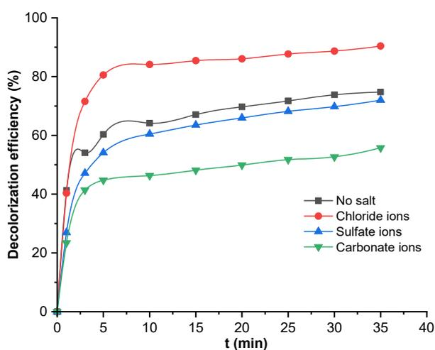
**Fig 7.** Effect of inorganic anions on PS decolorization. Experimental conditions: [PS] = 30 mg/L; [free chlorine] = 0.015 g/L; [inorganic anions] = 0.2 g/L; pH = 7
