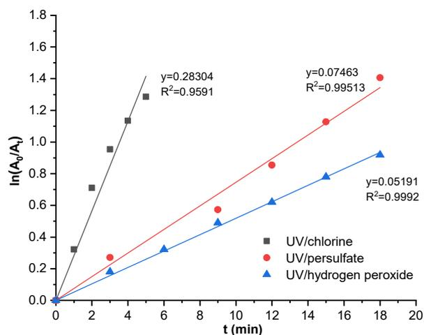
**Fig 3.** First-order plots for the PS degradation of PS at UV/chlorine, UV/S<sub>2</sub>O<sub>8</sub><sup>2-</sup> and UV/H<sub>2</sub>O<sub>2</sub> systems. Experimental conditions: [PS] = 0.044 mM; [H<sub>2</sub>O<sub>2</sub>] = [Cl(+I)] = [S<sub>2</sub>O<sub>8</sub><sup>2-</sup>] = 0.2 mM; pH = 7.75; T = 25 °C
