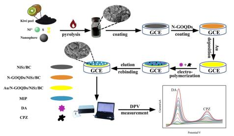
**Scheme 1.** Schematic of the preparation and electrochemical processes determination of the Au/N-GOQDs/NiS<sub>2</sub>/BC/MIP/GCE composite. Figure reproduced with permission from Author (Lu et al.); copyright from Elsevier [3]
