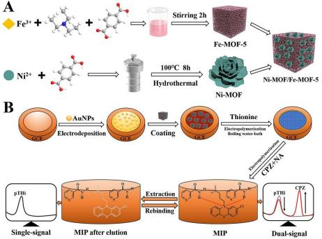
**Scheme 2.** Preparation procedure of (a) iron-metal organic framework-5 and nickel-metal organic framework and (b) MIP/pTHi/Ni-MOF/Fe-MOF-5/AuNPs on-off electrochemical sensor. Figure reproduced with permission from Author (Lu et al.); copyright from Elsevier [69]
