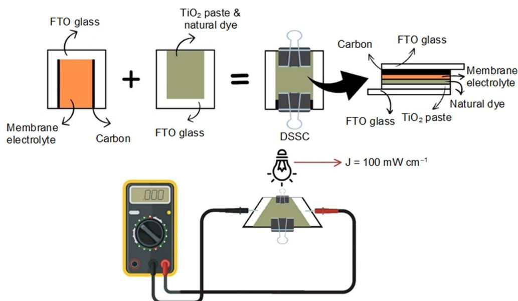
**Fig 1.** Diagram depicting the construction process of the DSSC
