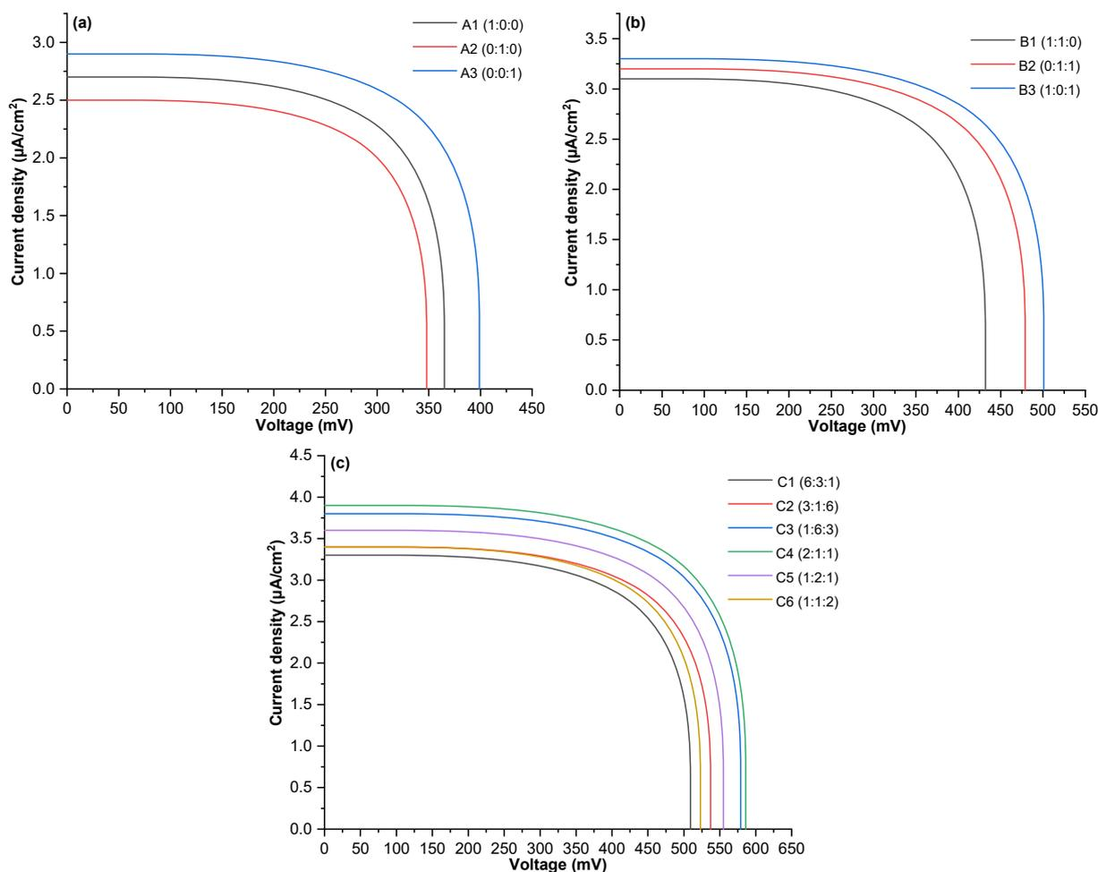
**Fig 4.** Photocurrent–voltage curves were obtained for DSSC sensitized of a) each single dye (red, yellow, and green), b) double blending of two dyes, and c) triple component blending of three dyes
