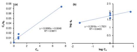
Fig 8. Linear graphs of (a) Langmuir and (b) Freundlich isotherms for Pb<sup>2+</sup> ion sorption by HAp/CTS 65 °C composite
