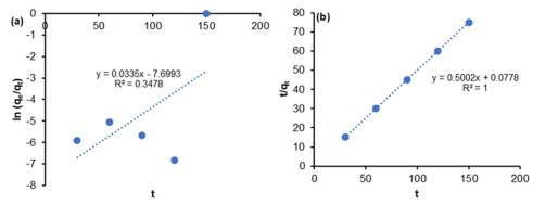
**Fig 9.** Linear graphs of (a) pseudo-first-order kinetics and (b) pseudo-second-order kinetics models on  $Cu^{2+}$  ion sorption by HAp/CTS 65 °C composite
