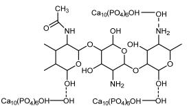
**Fig 3.** Proposed interaction between hydroxyapatite and chitosan [30]
