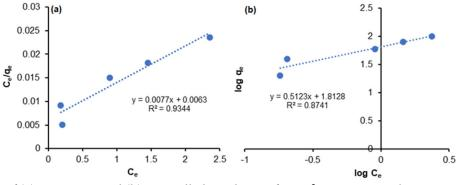
Fig 7. Linear graphs of (a) Langmuir and (b) Freundlich isotherms for Cu<sup>2+</sup> ion sorption by HAp/CTS 65 °C composite
