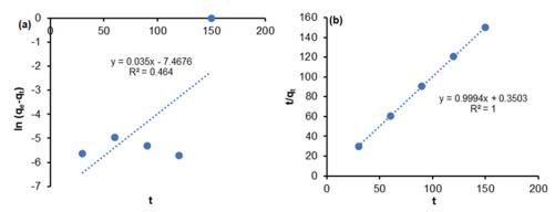
**Fig 10.** Linear graphs of (a) pseudo-first-order kinetics and (b) pseudo-second-order kinetics models on  $Pb^{2+}$  ion sorption by HAp/CTS 65 °C composite
