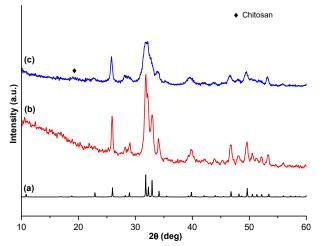
**Fig 4.** XRD spectra of (a) standard HAp, (b) cuttlefish bone HAp, and (c) HAp/CTS 65 °C composite
