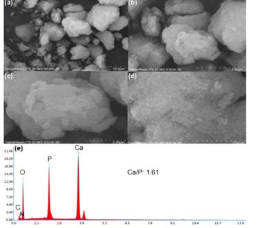
**Fig 5.** SEM photographs of HAp/CTS 65 °C composite: (a) 5,000×, (b) 10,000×, (c) 20,000×, and (d) 50,000× magnification and (e) EDS spectrum of HAp/CTS 65 °C composite
