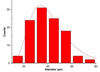
Fig 6. Particle size distribution of HAp/CTS 65 °C composite
