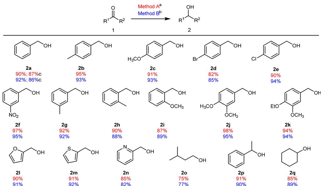
**Fig 1.** Scopes of reaction: a) reaction was carried out using grinding method at room temperature for 10 min; b) reaction was conducted under ultrasound irradiation at room temperature for 10 min, 40 kHz, 300 W; c) reaction was performed using 20 mmol of benzaldehyde
