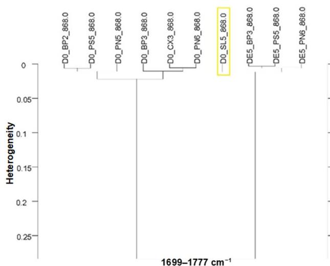
**Fig 4.** Dendrogram obtained from the HCA of raw spectra of B7 and B10 (10 spectra) partitioned into 2 main groups corresponding to two different types of biodiesel-diesel fuels. The clustering was performed between 1699 and 1777  $\text{cm}^{-1}$
