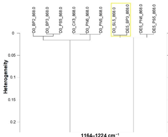
**Fig 5.** Dendrogram obtained from the HCA of raw spectra of B7 and B10 (10 spectra) partitioned into 2 main groups corresponding to two different types of biodiesel-diesel fuels. The clustering was performed between 1164 and 1224  $\text{cm}^{-1}$
