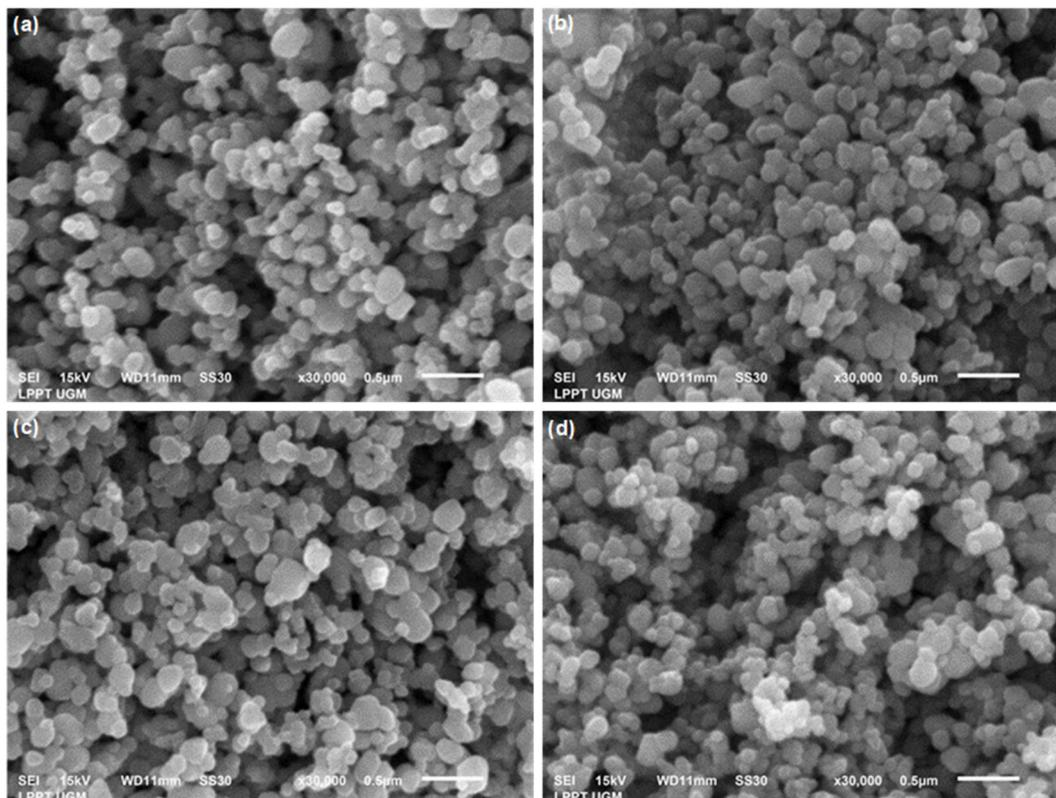
**Fig 6.** The SEM micrographs of (a) titanium dioxide, (b) titanium dioxide-Aceh curcuma 50 mg/L, (c) titanium dioxide-ethanol-curcumin 50 mg/L, and (d) titanium dioxide-triacetin-curcumin 50 mg/L composite materials
