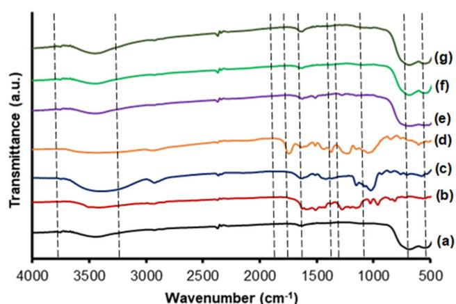
**Fig 5.** The FTIR spectra of (a) titanium dioxide, (b) Aceh curcuma, (c) ethanol-curcumin, (d) triacetin-curcumin, (e) titanium dioxide-Aceh curcuma 50 mg/L, (f) titanium dioxide-ethanol-curcumin 50 mg/L, and (g) titanium dioxide-triacetin-curcumin 50 mg/L composite materials
