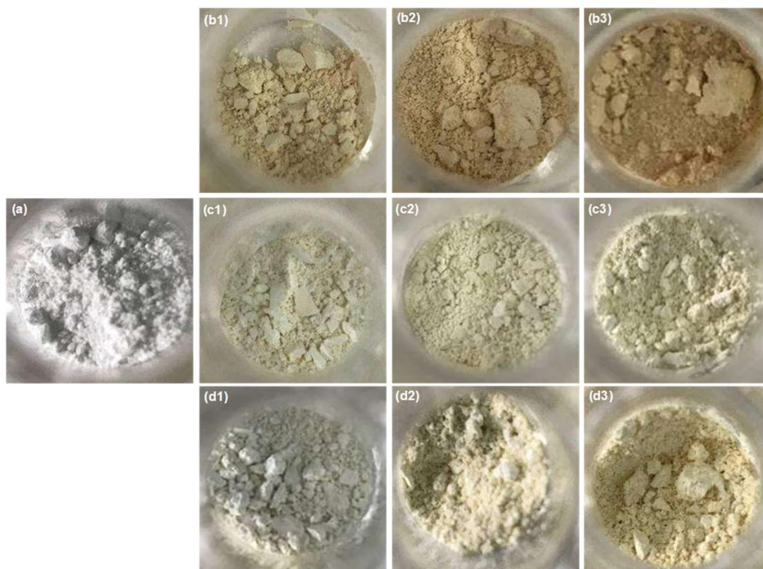
**Fig 2.** The photographed image of (a) titanium dioxide, (b1–b3) titanium dioxide-Aceh curcuma, (c1–c3) titanium dioxide-ethanol-curcumin, and (d1–d3) titanium dioxide-triacetin-curcumin composite materials. Terms (1), (2), and (3) stand for the initial concentration of curcumin solution of 5, 25, and 50 mg/L, respectively
