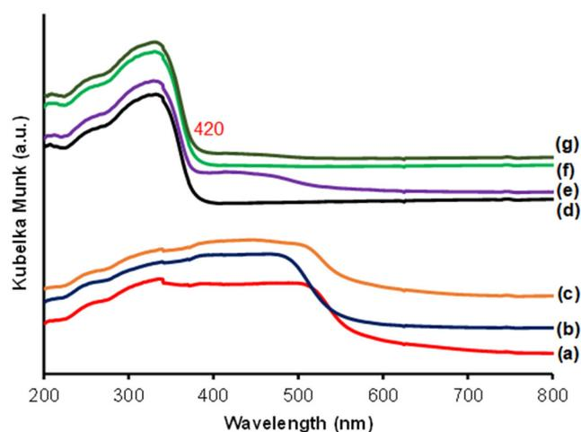
**Fig 3.** The DR UV-vis spectra of (a) Aceh curcuma, (b) ethanol-curcumin, (c) triacetin-curcumin, (d) titanium dioxide, (e) titanium dioxide-Aceh curcuma 50 mg/L, (f) titanium dioxide-ethanol-curcumin 50 mg/L, and (g) titanium dioxide-triacetin-curcumin 50 mg/L composite materials
