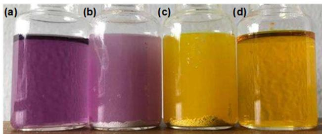
**Fig 9.** Photographed observation of DPPH solution (a) before and after the addition of (b) titanium dioxide, (c) titanium dioxide-curcumin composite material, and (d) Aceh curcuma as the antiradical agent
