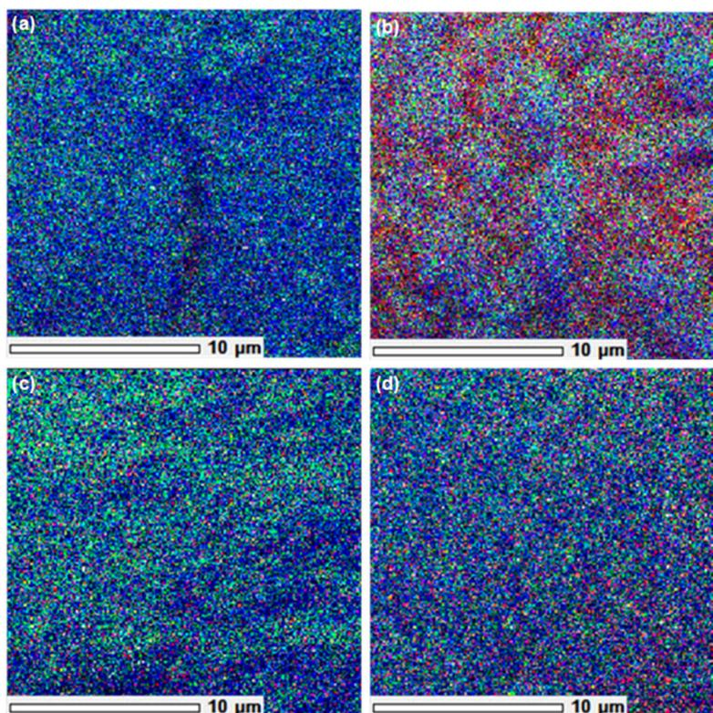
**Fig 7.** Elemental mapping of (a) titanium dioxide, (b) titanium dioxide-Aceh curcuma 50 mg/L, (c) titanium dioxide-ethanol-curcumin 50 mg/L, and (d) titanium dioxide-triacetin-curcumin 50 mg/L composite materials. Blue, green, and red colors represent titanium, oxygen, and carbon atoms
