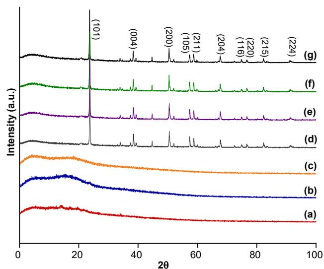
**Fig 4.** The XRD patterns of (a) Aceh curcuma, (b) ethanol-curcumin, (c) triacetin-curcumin, (d) titanium dioxide, (e) titanium dioxide-Aceh curcuma 50 mg/L, (f) titanium dioxide-ethanol-curcumin 50 mg/L, and (g) titanium dioxide-triacetin-curcumin 50 mg/L composite materials
