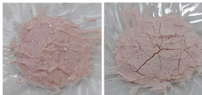
**Fig 1.** Paste (left) and cement (right) of HASiO<sub>2</sub>\_PE composite
