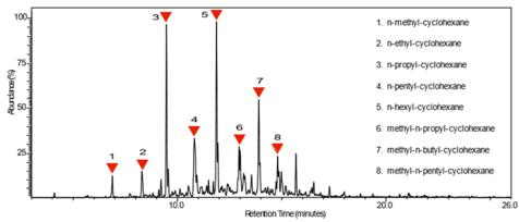
Fig S7. Fragmentogram m/z 83 showing the cycloalkane compound of Naphtha products
