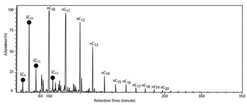
**Fig S4.** Fragmentogram m/z 57 showing n-alkane of naphtha products
