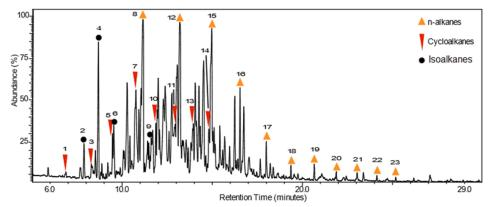
**Fig S1.** TIC of aliphatic hydrocarbon fractions of naphtha products that indicate the presence of *n*-alkane, isoalkane (branched alkanes), and cycloalkane compounds
