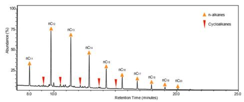
**Fig S2.** TIC of aliphatic hydrocarbon fractions of light oil (LO) products that indicate the presence of *n*-alkane and cycloalkane compounds
