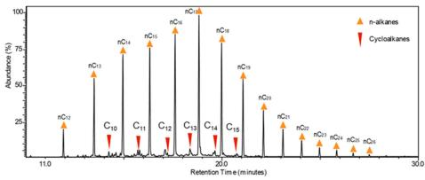
**Fig S3.** TIC of aliphatic hydrocarbon fraction of middle oil (MO) product which indicates the presence of *n*-alkane and cycloalkane compounds
