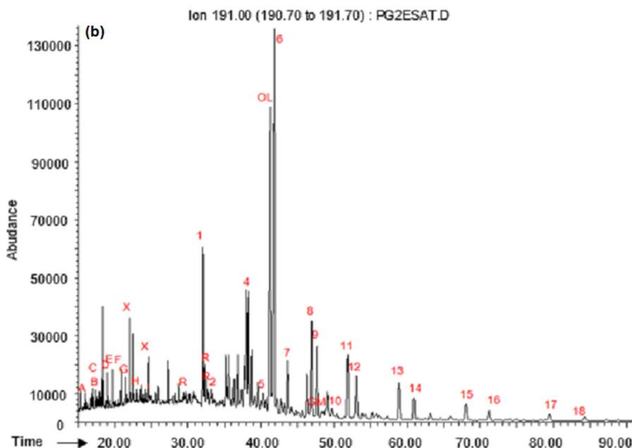
Fig 5. The mass fragmentogram of the terpene biomarker ( $m/z$  191) from (a) KK1 and (b) PG-02E
