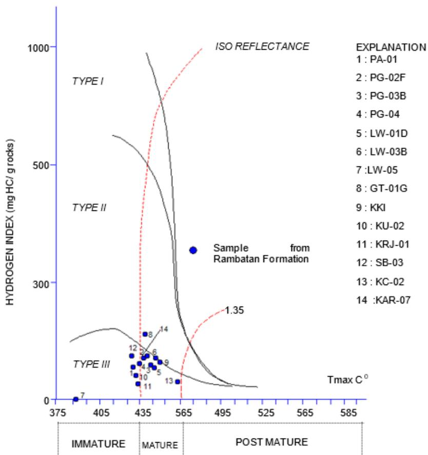
Fig 4. The plot of the HI vs.  $T_{max}$  for the Totogan and Rambatan Formation
