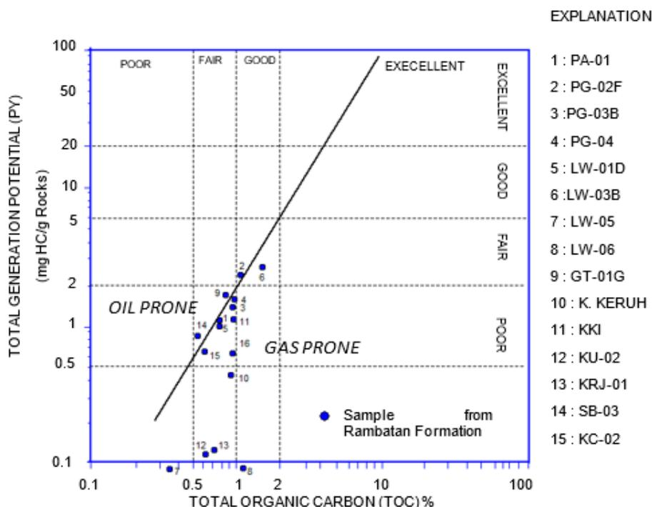
**Fig 3.** Diagram showing plotting Total Generation Potential Yield (PY) versus Total Organic Carbon (TOC) of The Totogan and Rambatan Formation
