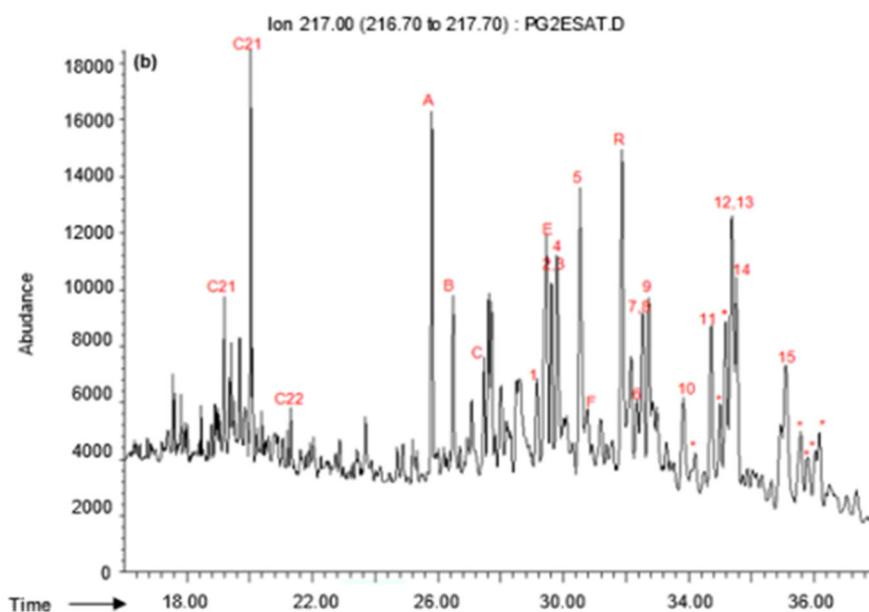
Fig 6. The mass fragmentogram of the biomarker sterane ( $m/z$  217) from (a) KK1 and (b) PG-02E
