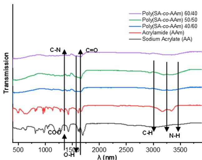
**Fig 2.** Fourier transform infrared spectra of sodium acrylate, acrylamide, and poly(sodium acrylate-*co*-acrylamide) (poly(SA-*co*-AAm)) samples prepared with sodium acrylate:acrylamide ratios of 40:60, 50:50, and 60:40
