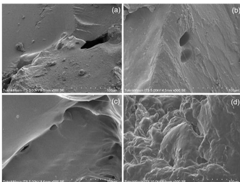
**Fig 1.** Scanning electron microscopy micrographs of poly(sodium acrylate-co-acrylamide) prepared with acrylic acid and acrylamide monomer ratios of (a) 40:60, (b) 50:50, and (c) 60:40 and (d) commercial flocculant Accofloc
