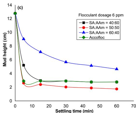
**Fig 4.** Effect of monomer concentration on the mud height upon addition of poly(sodium acrylate-*co*-acrylamide) dosage (a) 2 ppm, (b) 4 ppm, and (c) 6 ppm in comparison with commercial flocculant
