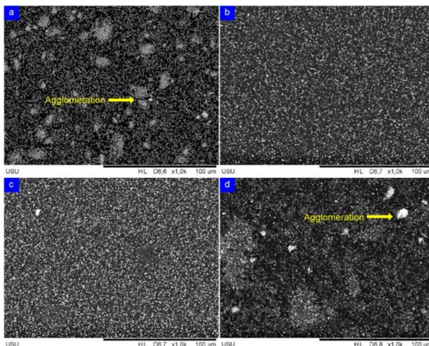
**Fig 2.** SEM images of (a) PVA/40TiO<sub>2</sub>/60SiO<sub>2</sub>, (b) PVA/60TiO<sub>2</sub>/40SiO<sub>2</sub>, (c) PVA/80TiO<sub>2</sub>/20SiO<sub>2</sub>, and (d) PVA/100TiO<sub>2</sub>/0SiO<sub>2</sub> composite membrane
