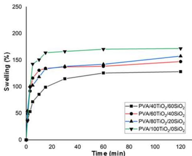
**Fig 5.** Swelling test of PVA/TiO<sub>2</sub>/SiO<sub>2</sub> composite membrane
