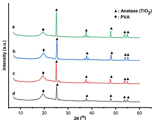
**Fig 4.** XRD patterns of (a) PVA/100TiO<sub>2</sub>/0SiO<sub>2</sub>, (b) PVA/80TiO<sub>2</sub>/20SiO<sub>2</sub>, (c) PVA/60TiO<sub>2</sub>/40SiO<sub>2</sub>, and (d) PVA/40TiO<sub>2</sub>/60SiO<sub>2</sub>
