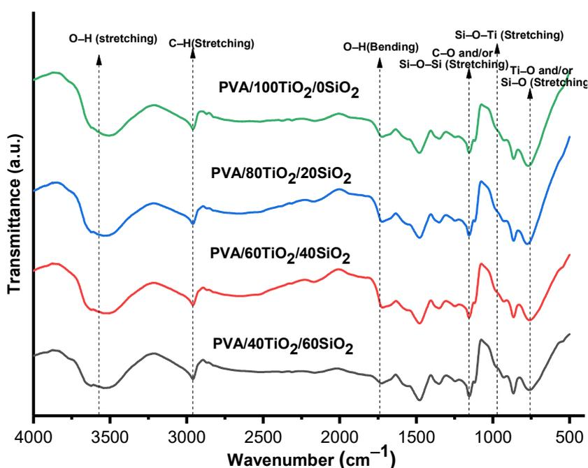
**Fig 1.** FTIR spectra of (a) PVA/40TiO<sub>2</sub>/60SiO<sub>2</sub>, (b) PVA/60TiO<sub>2</sub>/40SiO<sub>2</sub>, (c) PVA/80TiO<sub>2</sub>/20SiO<sub>2</sub>, and (d) PVA/100TiO<sub>2</sub>/0SiO<sub>2</sub> composite membrane
