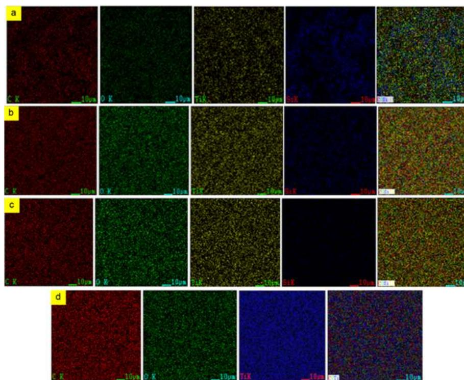
**Fig 3.** Elemental mapping of (a) PVA/40TiO<sub>2</sub>/60SiO<sub>2</sub>, (b) PVA/60TiO<sub>2</sub>/40SiO<sub>2</sub>, (c) PVA/80TiO<sub>2</sub>/20SiO<sub>2</sub>, and (d) PVA/100TiO<sub>2</sub>/0SiO<sub>2</sub> composite membrane
