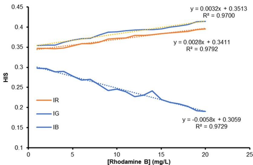
**Fig 5.** Calibration curve for  $(\text{RhB})_2\text{-Zn}(\text{CNS})_4$
