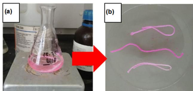
**Fig 3.** The extraction of rhodamine B from commercial red syrups using wool thread. Wool thread was dipped into the dissolved syrup residue for 10 min (a). Rhodamine B-containing wool thread before re-immersed to ethanol 70% and boiled (b)
